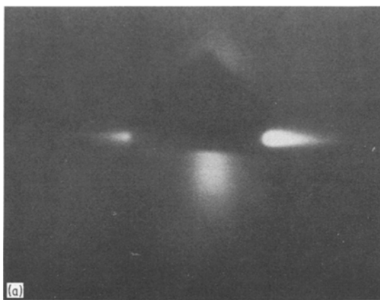
Figure 2 A typical SAXS pattern from crazes in a PS sheet under load. The insert shows the orientation of the craze fibrils which give rise to the vertical ( x -axis) fibril scattering streak. Longitudinal and circumferential line scans have the geometry shown, while the slit scan is performed by translating the slit shown along the x -axis. Because of the asymmetric parasitic scattering from the Kratky collimator the beam stop is elongated in the negative x -direction. Only the fibril scattering in the positive x -direction is analysed.
